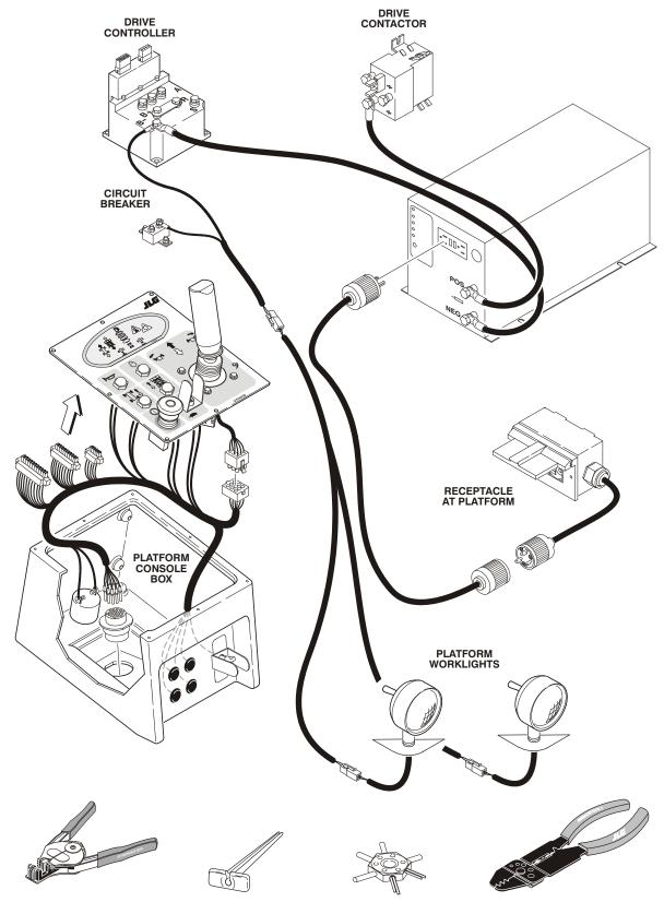
Figure 6-21. Electrical Components Installation - (Sheet 4 of 4)
