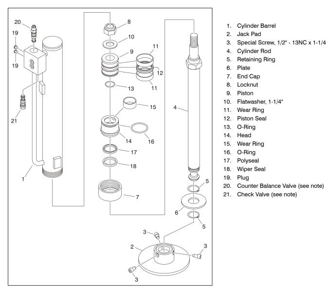
Figure 4-13. Leveling Jack Cylinder
