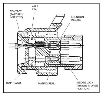
Figure 6-6. Connector Assembly (1 of 4)
