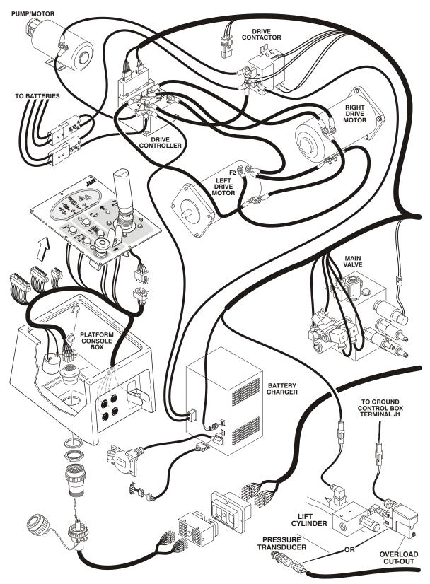
Figure 6-18. Electrical Components Installation - (Sheet 1 of 4)
