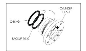
Figure 4-7. Installation of Head Seal Kit (Typical)
