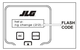
**NOTE:** Diagnostic Trouble Codes (DTC's) will only show for machines with software P1.0 and above. The 3 to 5 digit DTC will display in parenthesis on the JLG Analyzer in the upper right corner of the display screen as shown below. Refer to Table 5-1 for DTC's.
