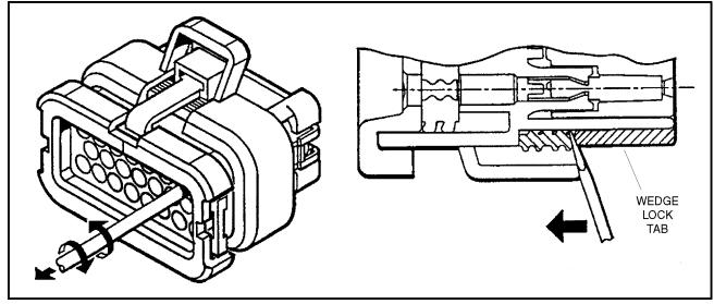
Figure 6-10. Connector Disassembly
