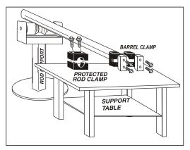
Figure 4-1. Barrel Support
