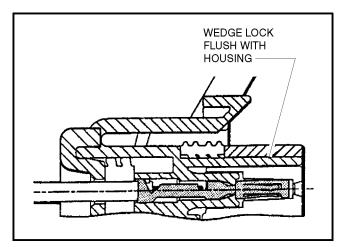
Figure 6-9. Connector Assembly (4 of 4)
