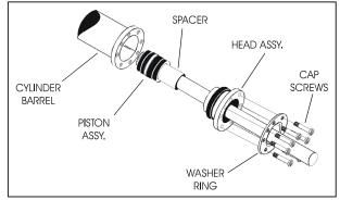
Figure 4-10. Rod Assembly Installation
