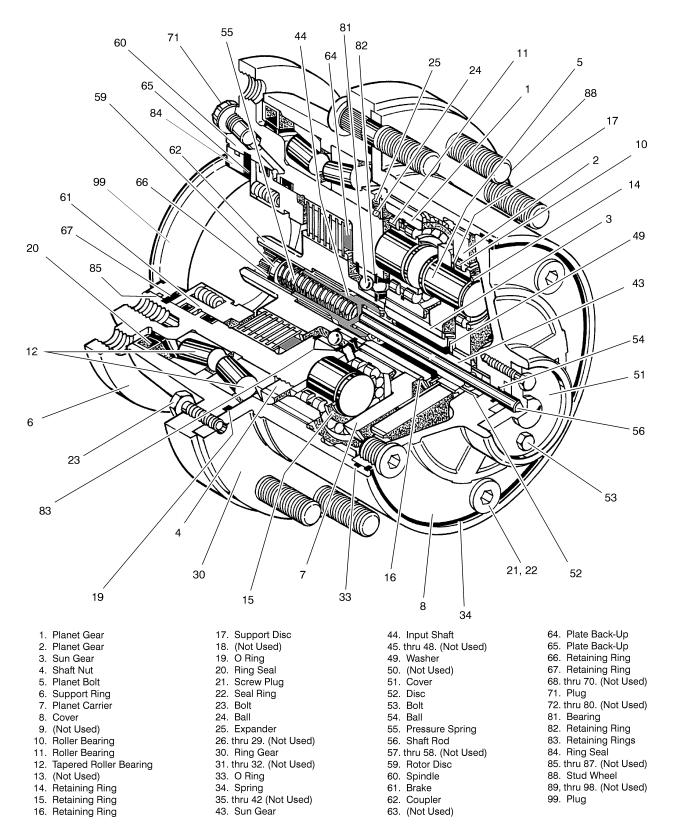
Figure 3-14. Torque Hub
