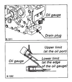
Kubota OC60-D Engine - Oil Dip Stick and Drain Location
