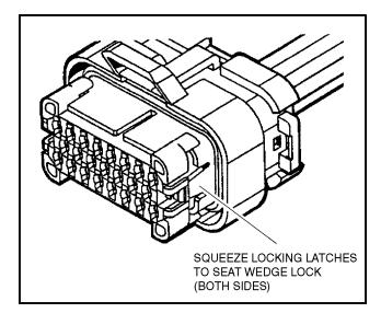
Figure 6-8. Connector Assembly (3 of 4)
