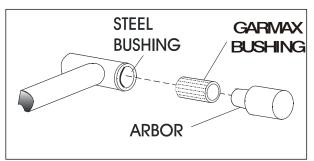
Figure 4-4. Oil-lite Bearing Installation
