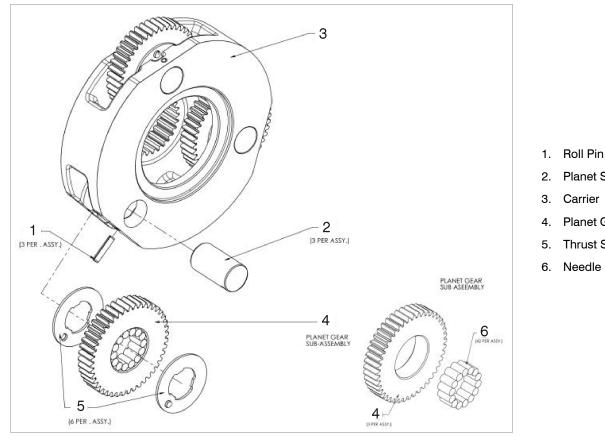
Figure 3-23. Input Carrier Sub-Assembly
