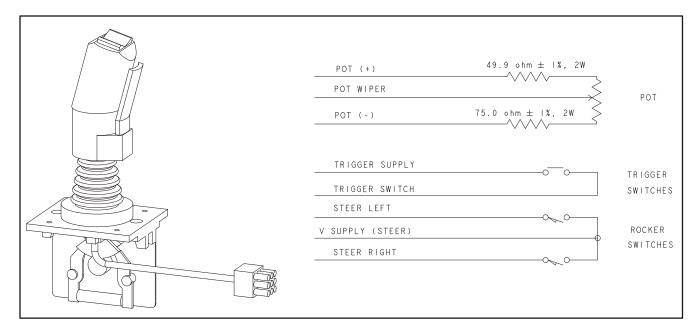
Figure 3-11. Joystick Controller - (JLG P/N 1600403)
