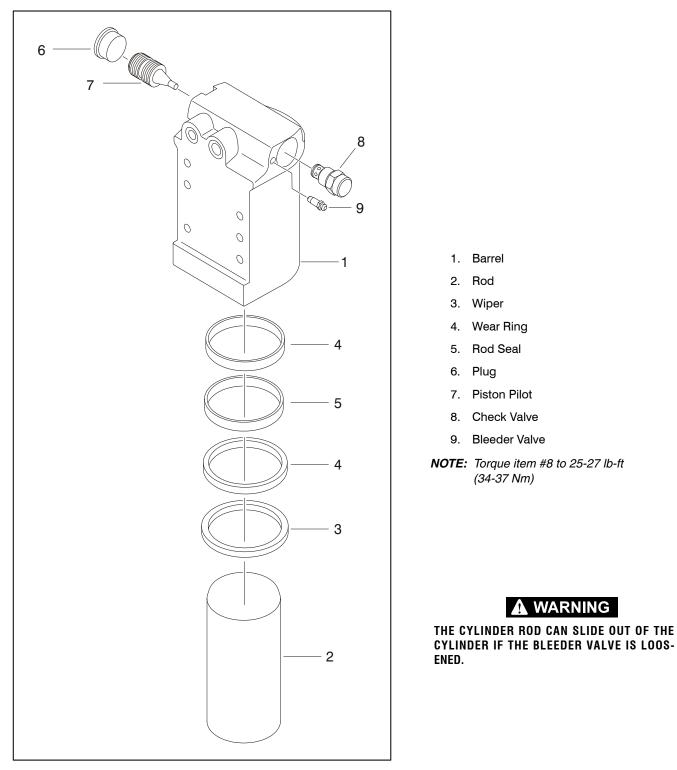
Figure 4-17. Oscillating Axle Cylinder
