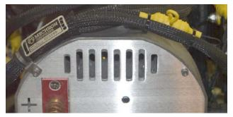
7. Reconnect the lift and APU start battery. The APU is now ready for use.
