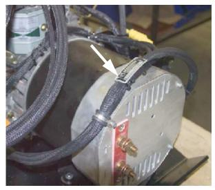
2. Find where the harness attaches to the rear cover of the generator and the connection point for the new inline fuse.
