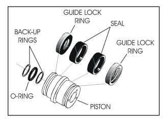
Figure 4-8. Piston Seal Kit Installation (Typical)
