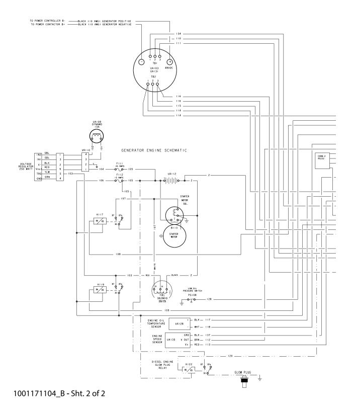
Figure 6-24. Electrical Schematic - Kubota (T4F) - Generator Only - Sheet 2 of 2
