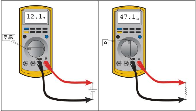
Figure 6-1. Voltage Measurement (DC)
