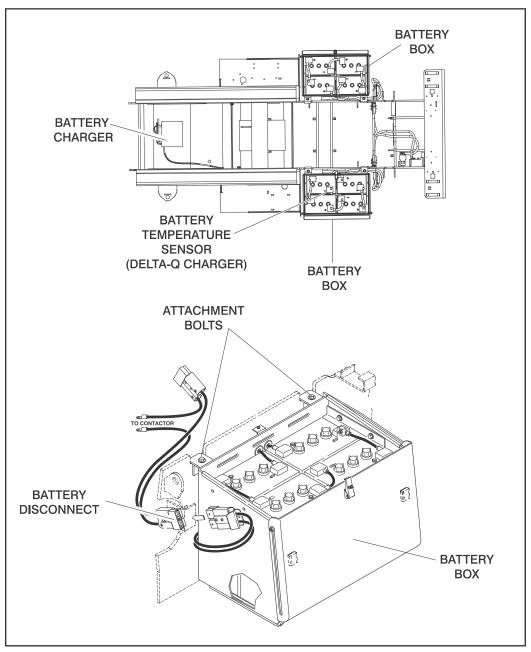
Figure 3-8. Batteries and Battery Charger
