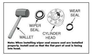
Figure 4-6. Wiper Seal Installation
