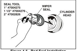
Figure 4-5. Rod Seal Installation
