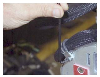
4. Cut and remove the Wire Ties holding the Harness label to the harness. Next, remove the Wire Ties so that the cable sleeve can be moved, exposing the conductors of the harness.
