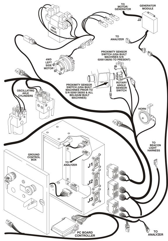
Figure 6-19. Electrical Components Installation - (Sheet 2 of 4)
