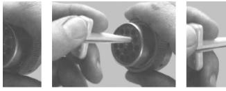
Figure 6-16. HD/HDP Contact Removal
