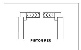
Figure 4-9. Poly-Pak Piston Seal Installation
