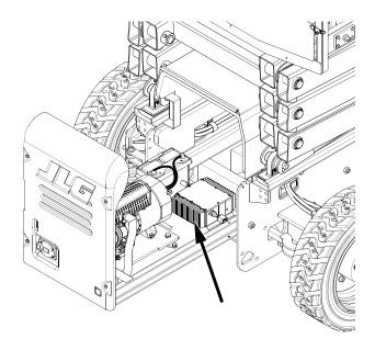
Figure 3-6. Battery Charger Location (M model shown)
