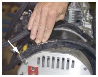
Remove the socket head drive screw with a 5/32" Allen key. Next remove the cable clamp from the harness.
